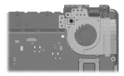
Where used: 1 captive screw that secures the fan to the base enclosure
